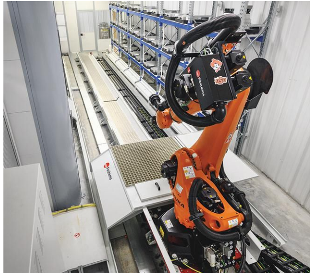
Advanced's 36-pallet system is connected to two Okuma MU 5000s and run by Fastems ROBO-One Flexible Manufacturing System (FMS).
