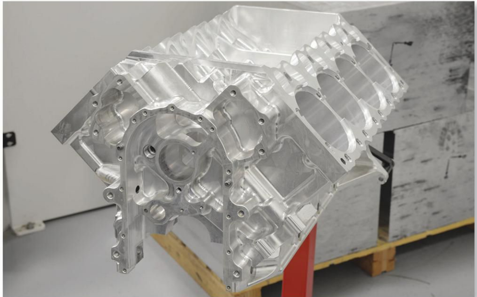
An engine block made in the manufacturing operations of Don Schumacher Racing. It started out as an 800 lb of aluminum and was machined down to 140 lb using high-speed Dynamic Motion and Opti-Rough Toolpaths to rough out complex geometries.
