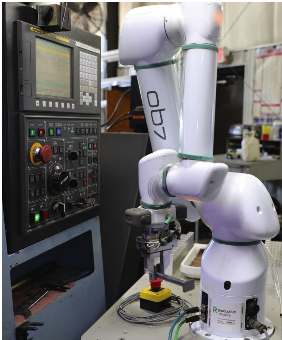
There were several compelling reasons why B.I.C. chose the OB7, however the top were: ease of use; "teaching" (versus programming); all-around flexibility from machine to machine; 7 axes rather than 6 (the OB7 is the only cobot on the market with the 7th axis "wrist" motion); the dedicated and responsive engineering; integration and service support they receive from Absolute Machine Tools; and that it is made in America.
