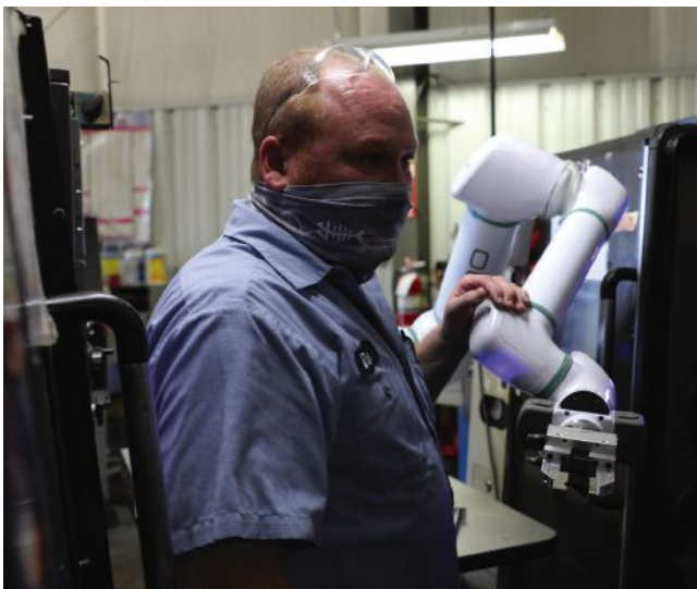
Cell and machine operator David Farris has become one of the resident experts on the cobot at B.I.C. Precision. Now he's free to work on less taxing and more interesting tasks in and outside the cell. He said the OB7's 7th axis J3 arm/wrist has allowed much greater maneuverability and flexibility in the cell.
