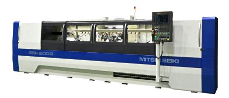
Mitsui Seiki's GSH 200A thread grinding machine combines flexibility of application, high processing speeds and consistent precision to complete an extensive selection of threading jobs, according to the company. The GSH 200A is engineered to handle a wide variety of workpiece sizes. Maximum diameter swing over the machine table is 480 mm and distance between centers is 2,250 mm, enabling the machine to grind a maximum screw length of 2,000 mm and maximum workpiece diameter of 200 mm.
