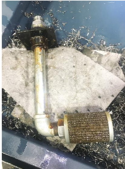
This is result of a shop not cleaning the oil reservoir tank and filter on a CNC machine tool. In this instance, the customer received a flow alarm, which had it not been caught in time, would have lead to a gear or bearing failure. (Provided by Absolute Machine Tools)
